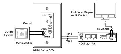
Figure 2-28 — Installation routing modulated IR
